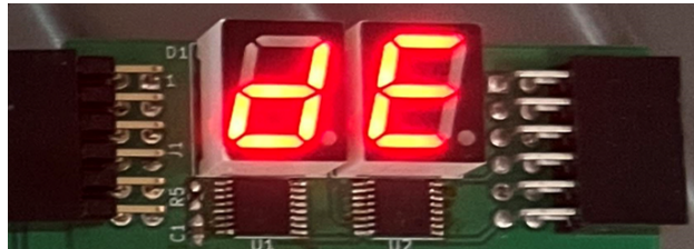
Figure 4.6 ChipForge Seven Segment Display PMOD
